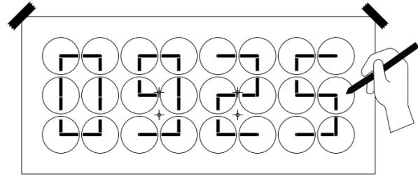
Drill the holes in the wall dimensioned to fit the wall anchors properly. Then, place the wall anchors and fix the hanging plate with the provided screws and washers.
