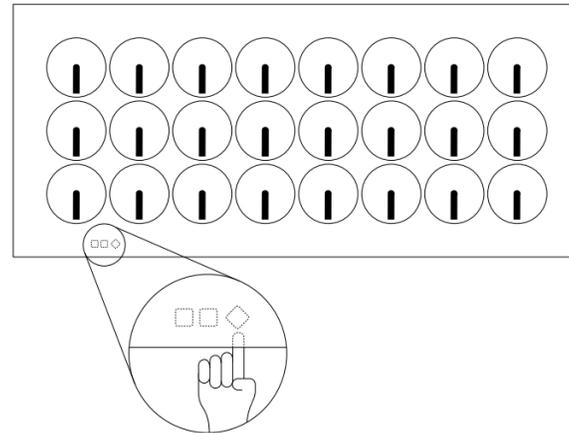
After starting the clock, the position of some clock hands might still need to be adjusted. In order to have the clock hands perfectly aligned with each other, you can fine-tune the clock hands' position by manually adjusting the clock hands while the time is displayed.
